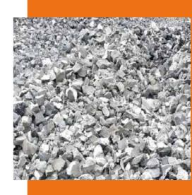
Our major manufacturing product is SYNTHETIC SLAG, which is a conditioner and is used as recovery increment of steel, grade improvement, to reduce the electricity consumption, for continuous casting of the slabs, to give strength and hardness to stainless steel, and it also provides a protective layer to prevent corrosion.
